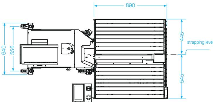
Frame size (650 x 600) with roller conveyor (990 x 890)
